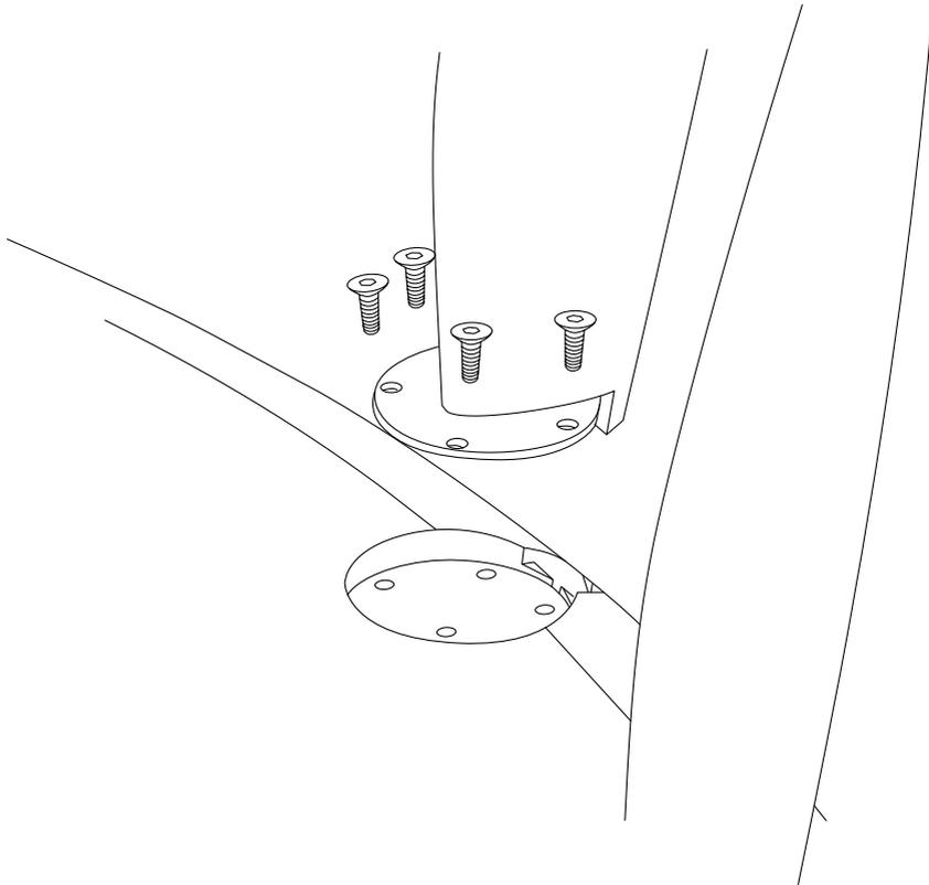
Screw four short screws for each leg. Repeat the process until all four legs are fixed to the table top.
